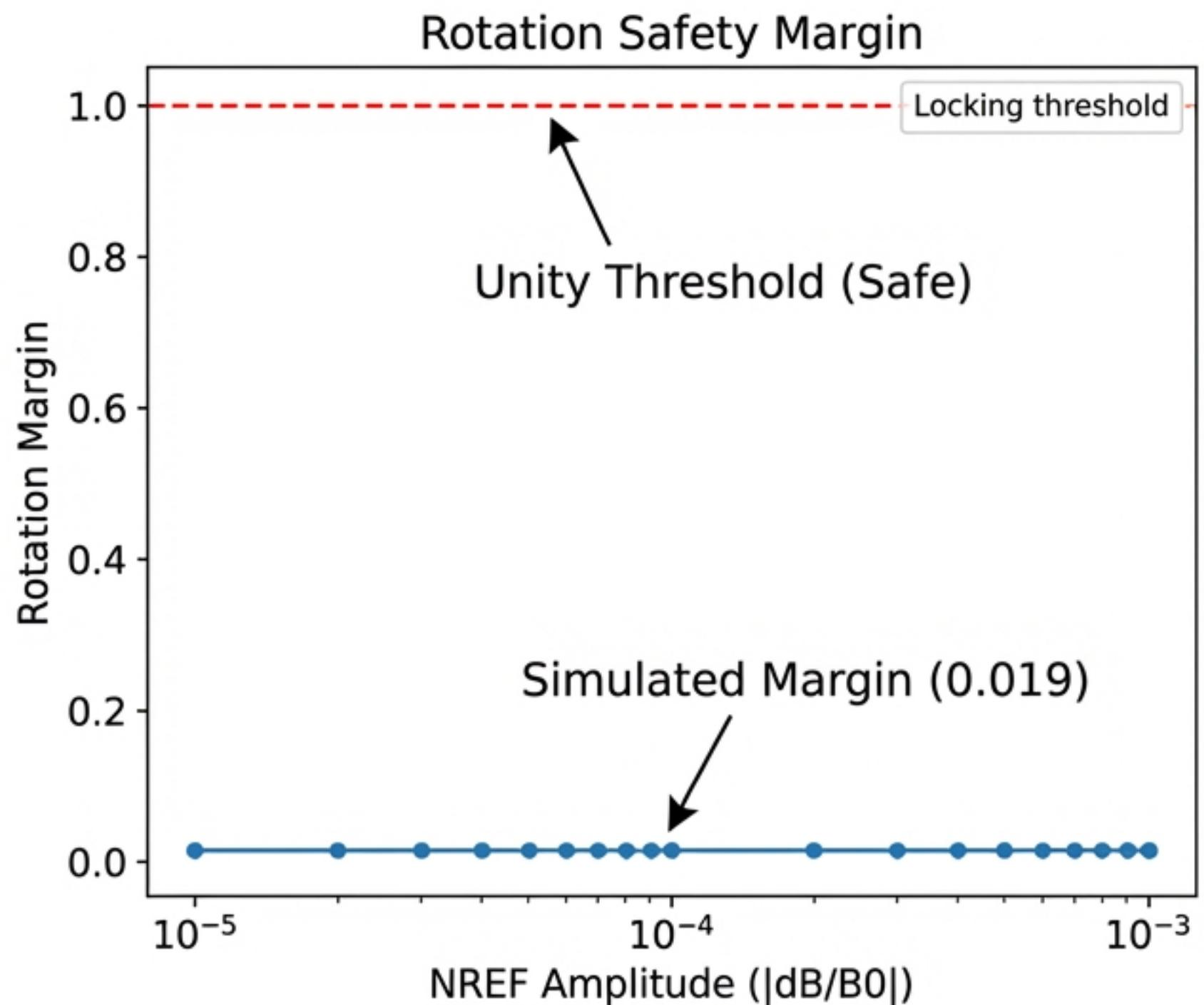
**The maximum correctable error field is capped at  $1.69 \times 10^{-4}$  relative to  $B_0$ .**
